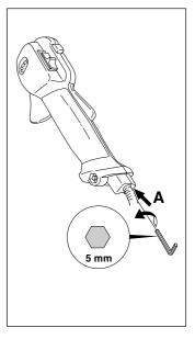
CAUTION! Contact your servicing dealer, if the idle speed setting cannot be adjusted so that the cutting attachment stops. Do not use the machine until it has been properly adjusted or repaired.
